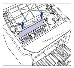
☐ If the jam is difficult to clear, pull the paper out from the multi-purpose tray or manual feed tray.
